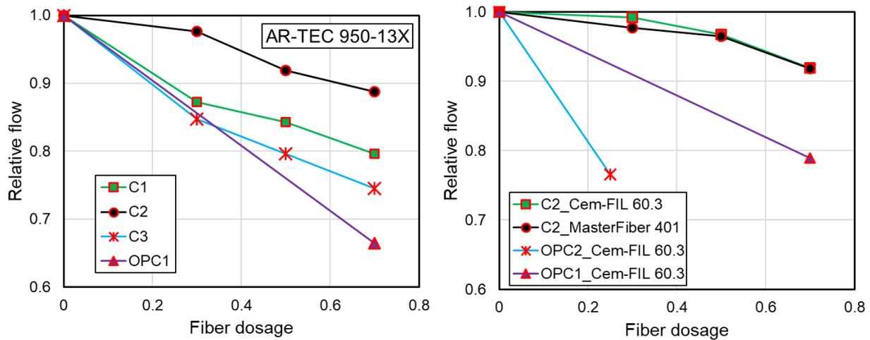
Fig. 2. Relative flow vs. fiber dosage
