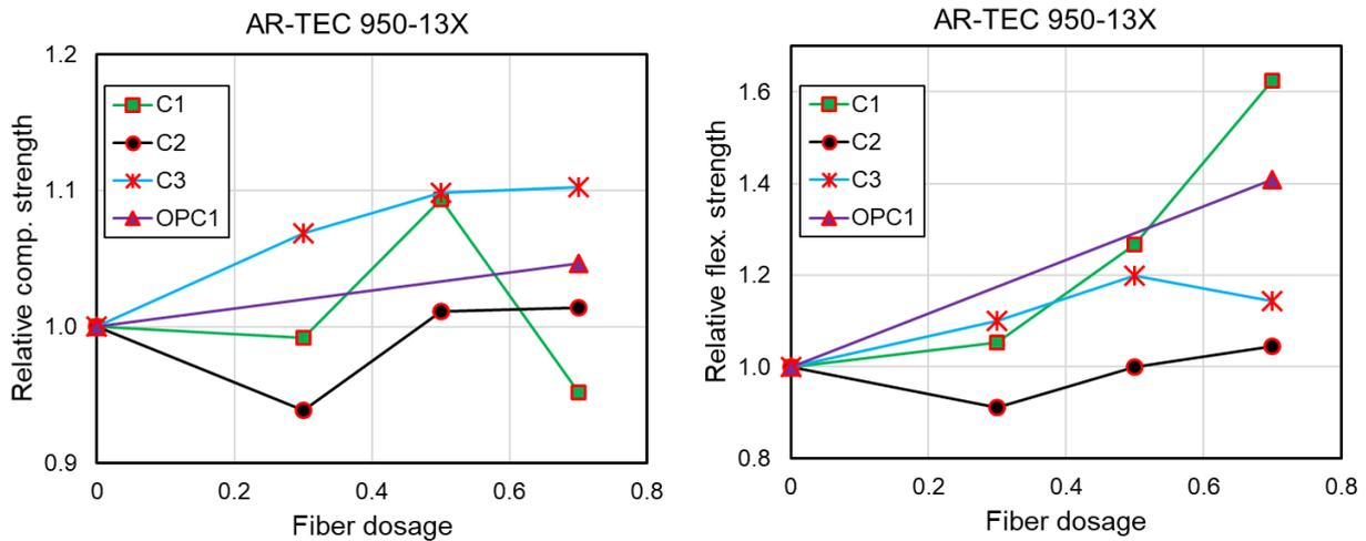
Fig. 3. Relative compressive and flexural strengths
